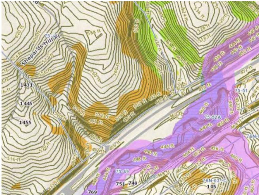
Figure 10: Critical Slopes on Northwest Side of U.S. 29
